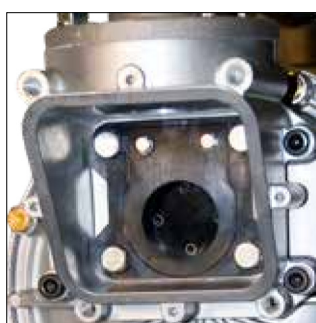
Only 4 bolts to access flap valves
