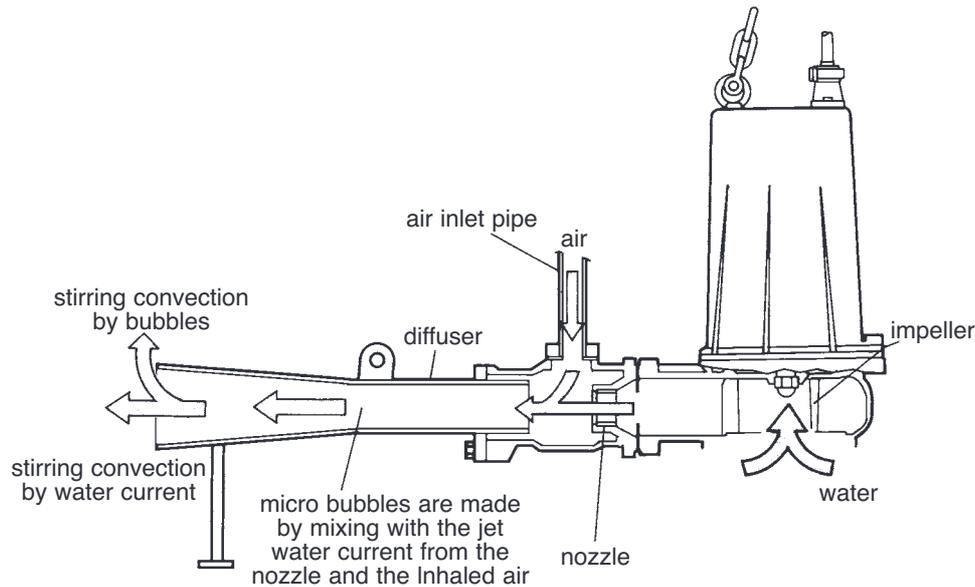
The Tsurumi Submersible Ejector, as shown in the figure, draws air in from around the jet nozzle (venturi) by means of the water power discharged from the submersible pump.
