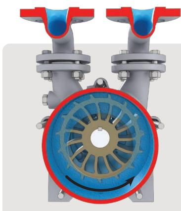
Simplified diagram of liquid ring pump and compressor operation
